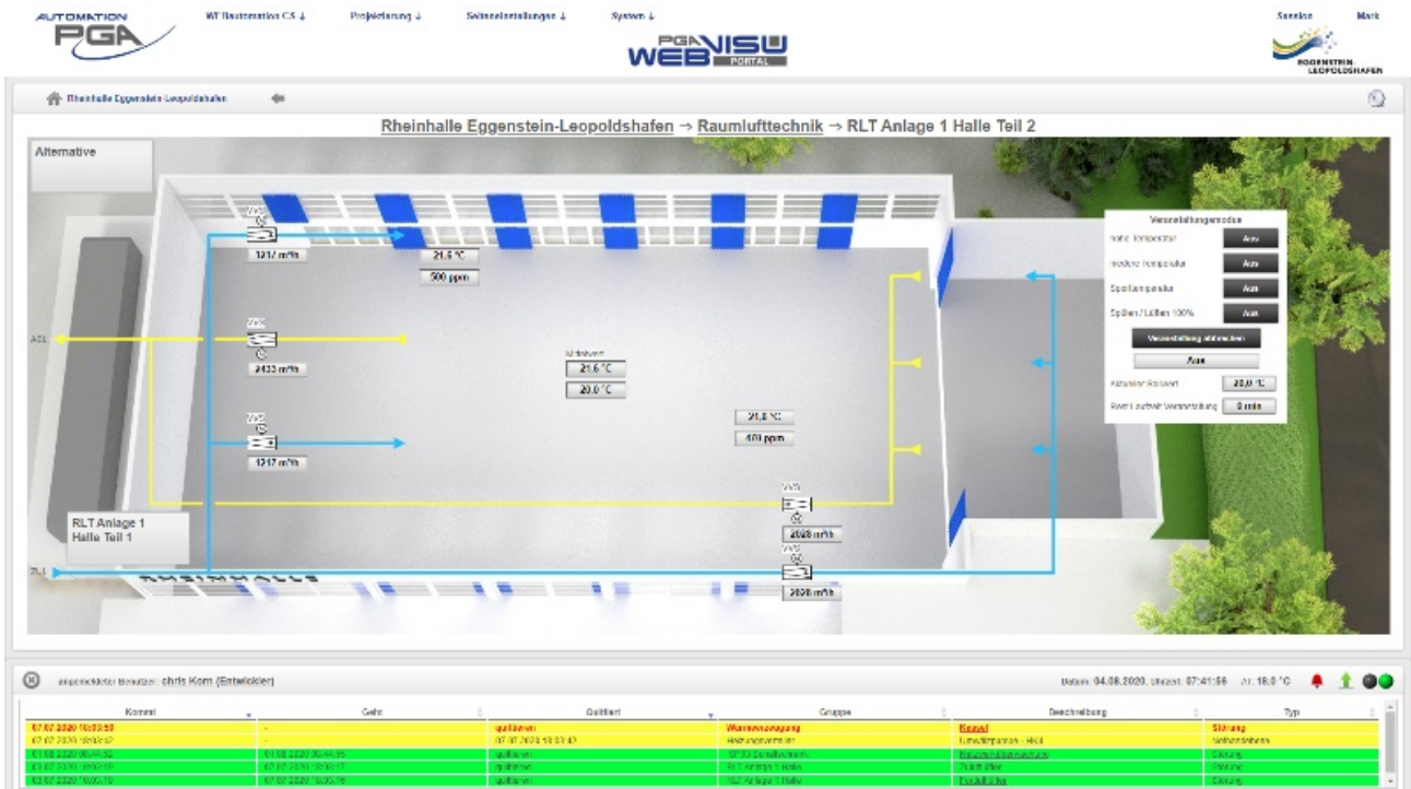
Figure 6 Air handling unit AHU system 1 hall part 2
