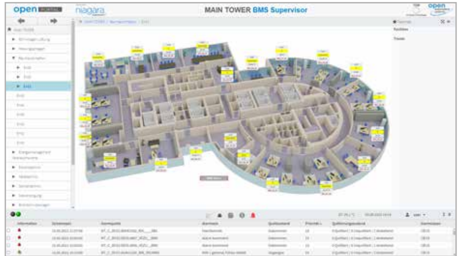
OAS BMS Supervisor MAIN TOWER – Floor View.
